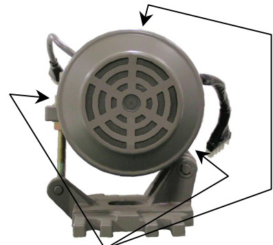
End cover mounting screw
